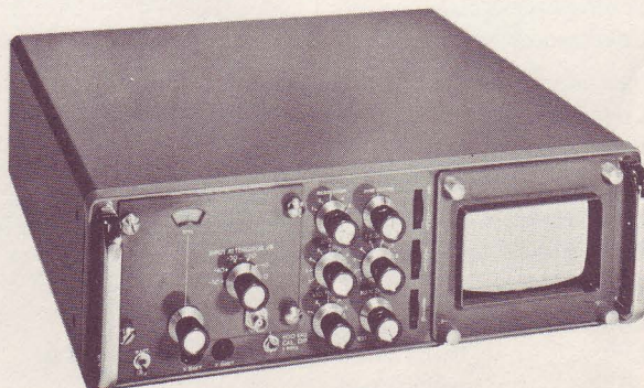
Frontal appearance of Model EP961 Panoramic Display Unit
